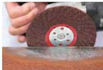
Rust, coating, glue, mastic removal
